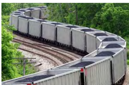
Figure 4. One coal car carries approximately 110 tons of coal which roughly produces 2300 kwh
